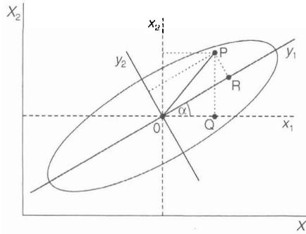
**Figure 4.** Principal component analysis. The diagram shows the contour ellipse of a bivariate distribution with its centroid at the point labeled  $O$ . The centered coordinates  $x_1$  and  $x_2$  are derived from the original variables  $X_1$  and  $X_2$  by subtracting their mean values. The principal components  $y_1$  and  $y_2$  are the directions of maximal and minimal variance, respectively. See text for details.
